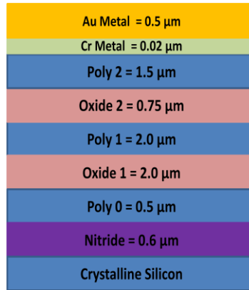
Figure 64. A schematic illustrating the layers and their corresponding dimensions used in the polyMUMPS ® process.
